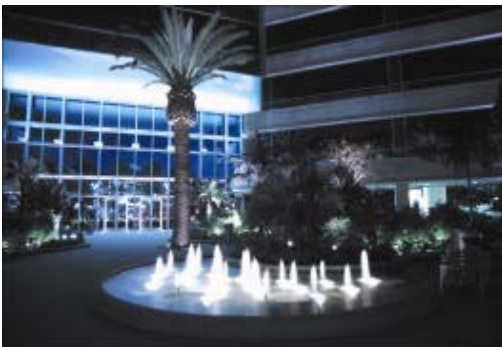
Figure 6.4 – Uplighting can be used to indirectly illuminate entries if layout doesn't cause light pollution.
