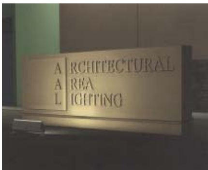
Figure 10.2 – Where sign lighting is uplighted, barn doors, louvers, and other accessories can minimize light pollution.
